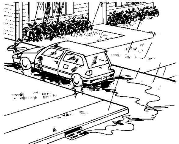
are toxic to downstream aquatic life. Downspouts positioned to empty directly onto driveways compound the problem.
